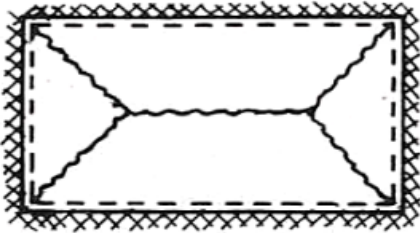
Rectangular slab (fixed supports)
